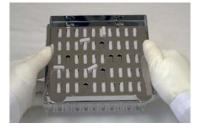
**1.** Pour 50+ trial capsules onto the Orienter. Shake back and forth moving them into the slots.
