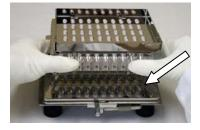
**3.** Place the Orienter locating feet into the holes further away from the operator on sheet "c".
